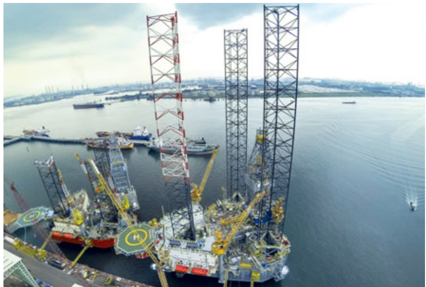
Keppel FELS delivered its first four KFELS Super A Class jackups in 2013, two each to Hercules Offshore and Ensco. They can work in harsh environments of the North Sea and other parts of the world.
