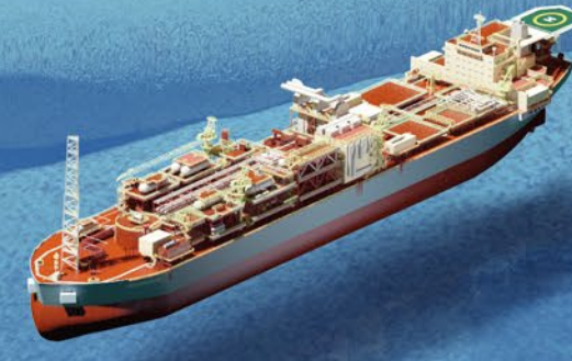
▶ Floating Production Storage and Offloading Facility (FPSO)
