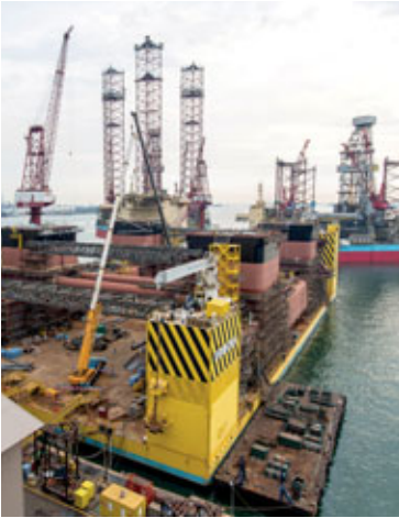
The CAN-DO barge at Keppel FELS has increased the yard's capability to take on bigger projects like the construction of the hull of the DSS™ 38E semi for Brazil.
