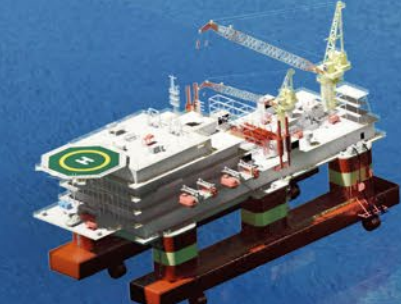
▶ Semisubmersible Accommodation Unit (SSAU)
