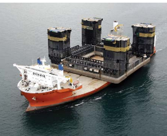
The lower hull of P-52 rests on Blue Marlim – a dry-tow vessel – as it sets sail for Brazil
