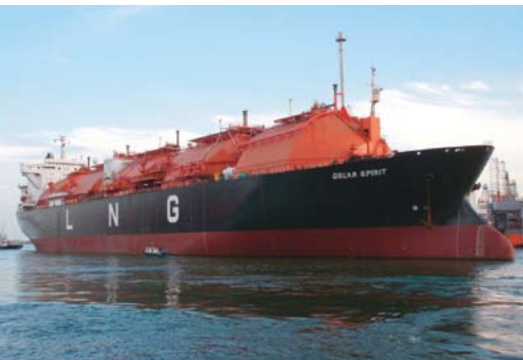
Golar Spirit , the world's first LNG re-gasification unit was converted at Keppel Shipyard
