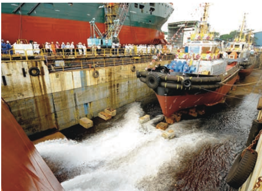
The drydock was flooded for the launch of three tugboats for Keppel Smit Towage and Port of Salalah
