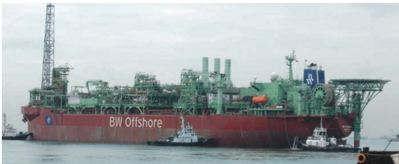
BW Pioneer on its way to the US Gulf of Mexico, where it will be the first FPSO deployed there
