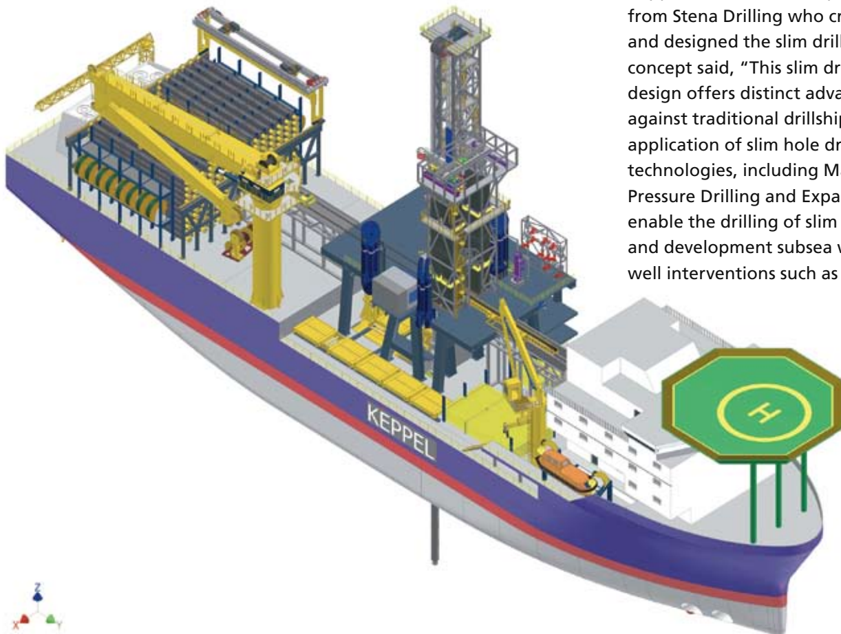
KOMtech's slim drillship is a safe, economical and technologically-advanced solution for re-entry into existing subsea wells
