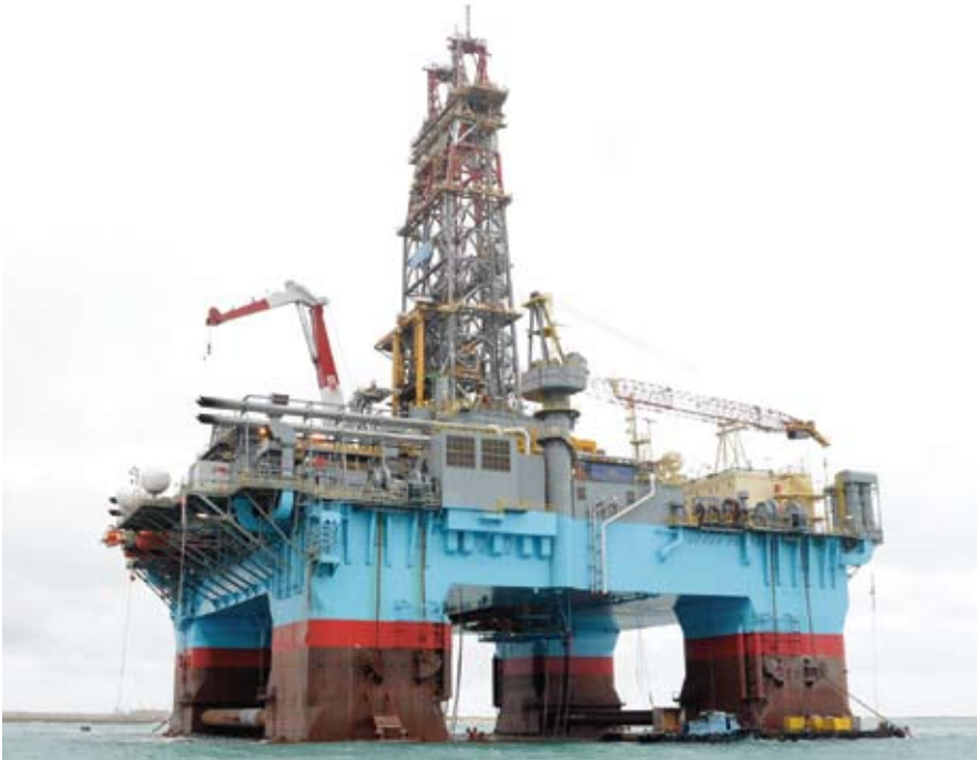
DSS™ Series rigs are highly cost effective exploration units capable of drilling down 10,000 m (30,000 ft) wells and operating at a water depth of 3,000 m (10,000 ft). The Series also features a dynamic positioning system, with the ability to attach to a pre-laid mooring system
