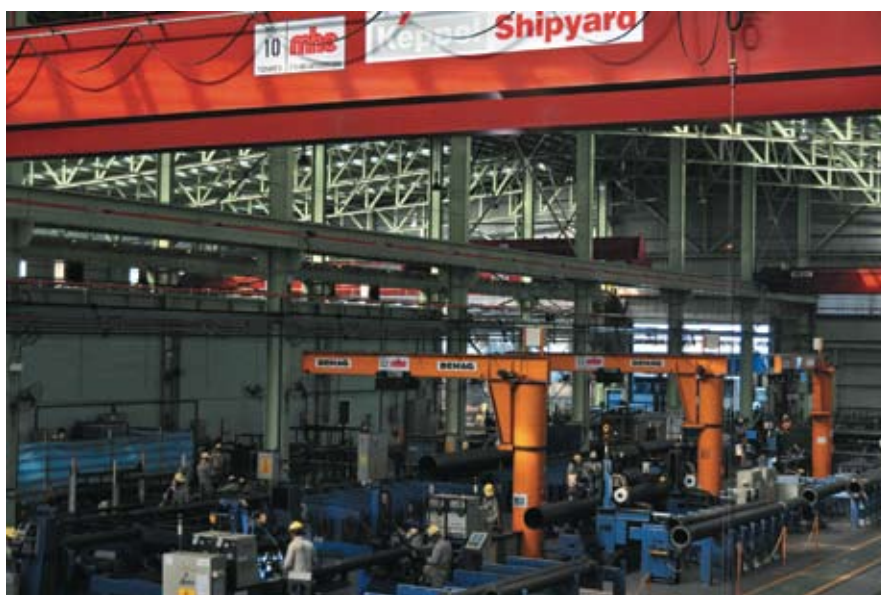
The semi-automated pipe shop has boosted productivity of pipe fabrication by 45% at Keppel Shipyard
